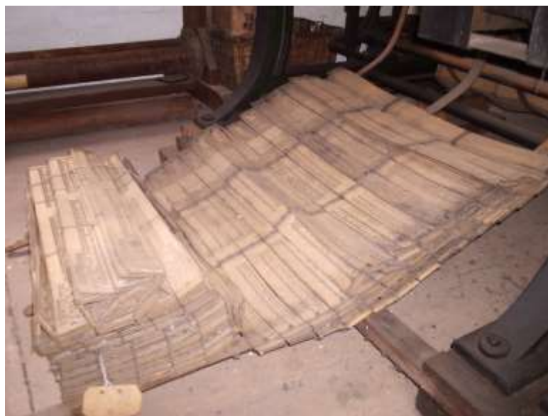
Rolls of punch cards – Jacquard system of lace production (Wollaton Museum)
